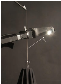
Fig. 7. The gantry setup used to measure the BxDF of threads. The thread is suspended vertically, which makes it possible to capture the full 4D BxDF.
